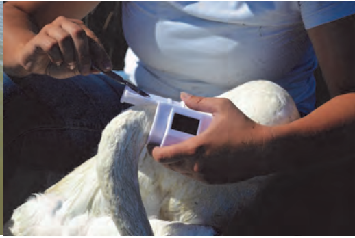
Attaching the lightweight Ornitela GSM collars. The collars have solar panels and battery packs, with an expected life of 3 years.
