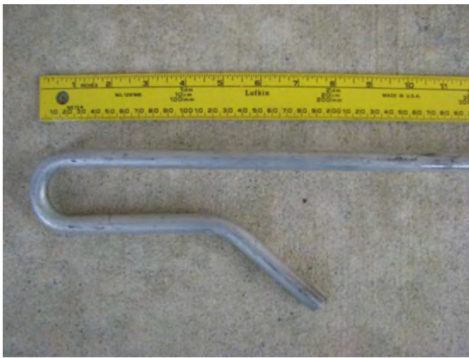
Figure 1. Distal end of telescopic, aluminium swan pole (3.2-cm crook gap) made of marine-grade aluminium rod (0.6 cm) used to capture flightless mute swans in the lower Potomac River and upper Chesapeake Bay, Maryland, USA, 2005–2008.
